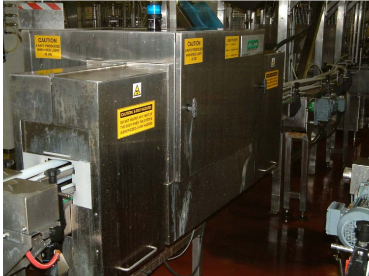
The x-ray system installs immediately after the seamer in tight space here as shown in a vegetable canning application. [Note: Rear of inspection assembly is shown.]
